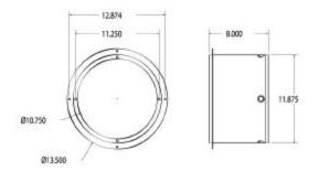
ENCLOSURE FROM 22 GA CRS (PRIMER) ENCLOSURE PROVIDED WITH 4 EA. 8-32 J NUTS KNOCK OUTS SHOWN 1/2" AND 3/4" COMBINATION
